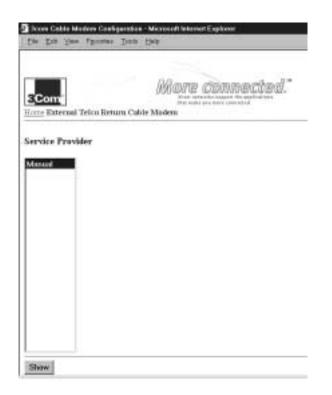
Access this screen to enroll into a new cable modem access account with a Broadband Service Provider (BSP).
